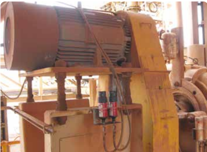
Application Electric motor with reverse overhead configuration driving a horizontal slurry pump Lubricator perma STAR VARIO L250 Installation kit K230C
