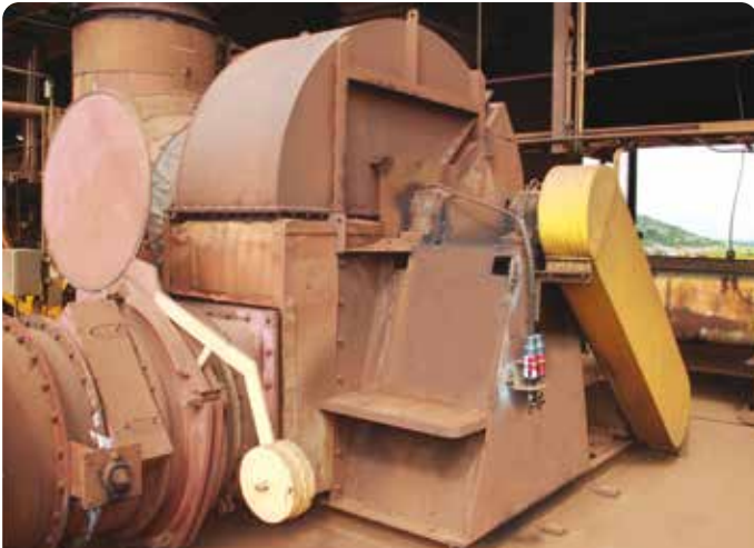
Application Fan support bearings Lubricator perma STAR VARIO L250 Installation kit K230C
