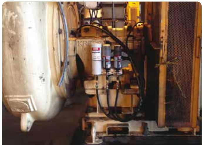
Application Horizontal slurry pump labyrinth seals and gland seal Lubricator perma STAR VARIO L250 Installation kit K365C
