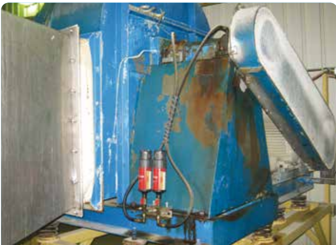
Application Fan support bearings Lubricator perma STAR VARIO L250 Installation kit K230
