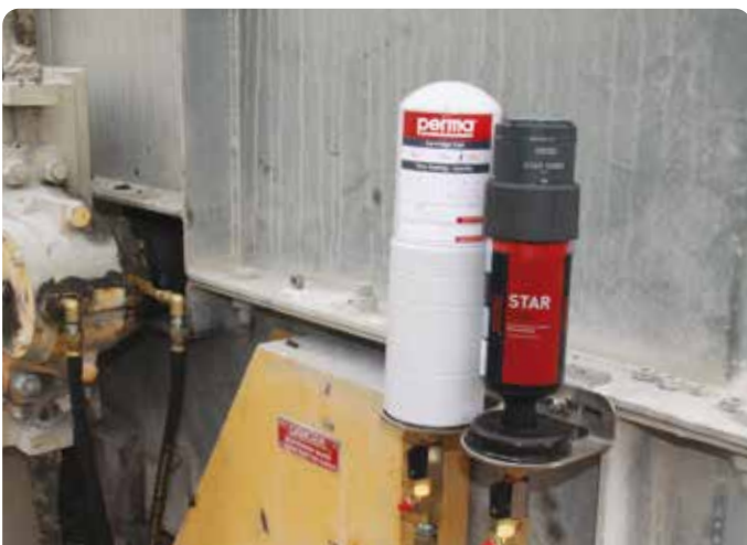
Application Conveyor pulley bearing and seal Lubricator perma STAR VARIO L250 Installation kit K230
