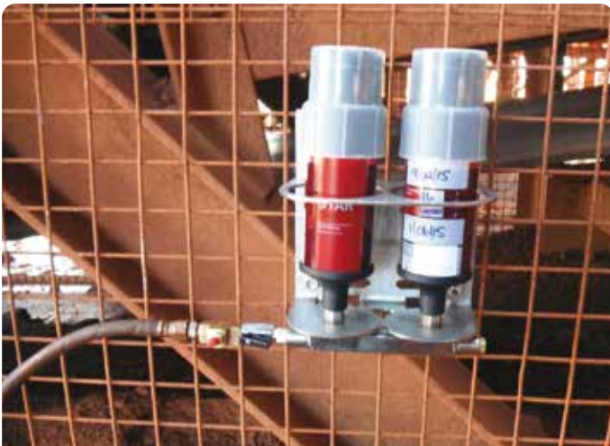
Application Conveyor pulley seals – this is a hybrid solution where the relubrication of the bearings is performed manually Lubricator perma STAR VARIO L250 x 2 Installation kit K2CHCJ
