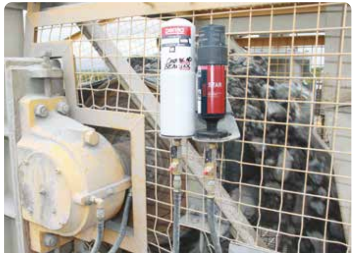
Application Conveyor pulley bearing and seal Lubricator perma STAR VARIO L250 Installation kit K2CH
